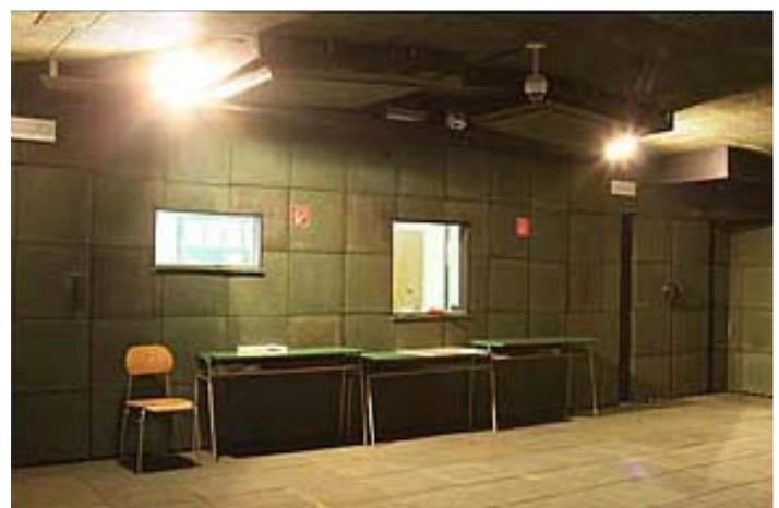
Big bullet-proof window to control room, first transverse ramp with the stroboscopic lights, adjustable lights, dome video camera and air-conditioning output. Audio system in the corner up.
