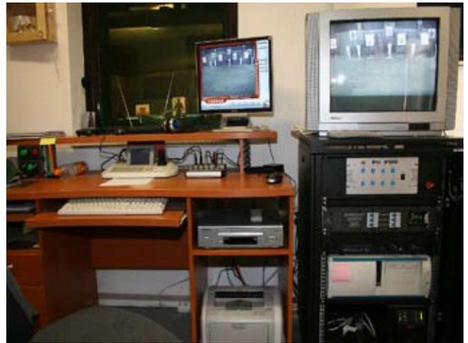
Rack with electronics equipment for control and programming scenes with lights, stroboscopes, smoke machines, sound effects etc.
