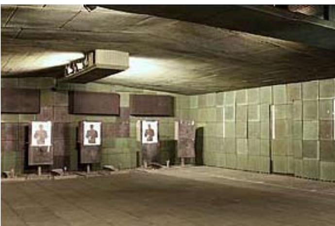
Up in front 2nd transverse ramp with the device for smoke machine, stroboscope and adjustable lights. In the back you can see the third ramp with lights and stroboscopes. In right wall between two white lines you can see closed entrance door for shooters
