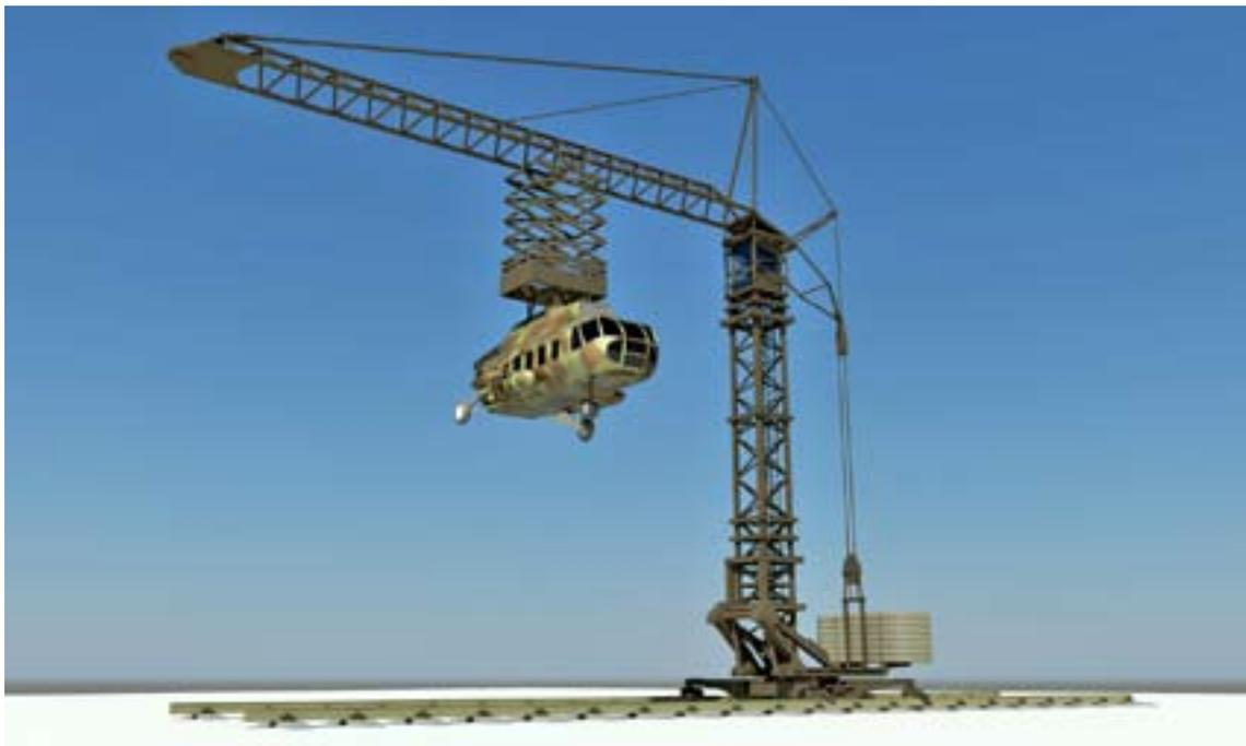
**SECTION B:** The helicopter module is a copy of a real chopper fuselage. The flight cabin is identical with the chosen type of helicopters. There are all important items necessary for functions and for creating a real environment for the crew making authentic optical and tangible impact on the crew's psyche.
